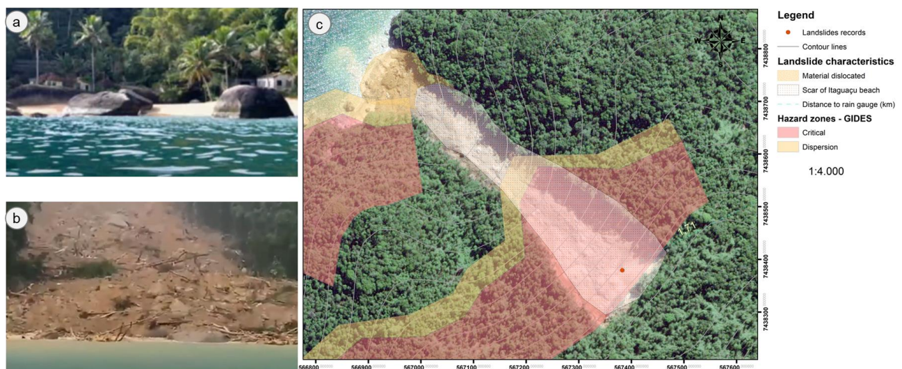
Figure 3. High-magnitude shallow translational landslide of the Itaguaçu Beach: a-b) before and after the event, c) hazard mapping according to the GIDES procedures.
