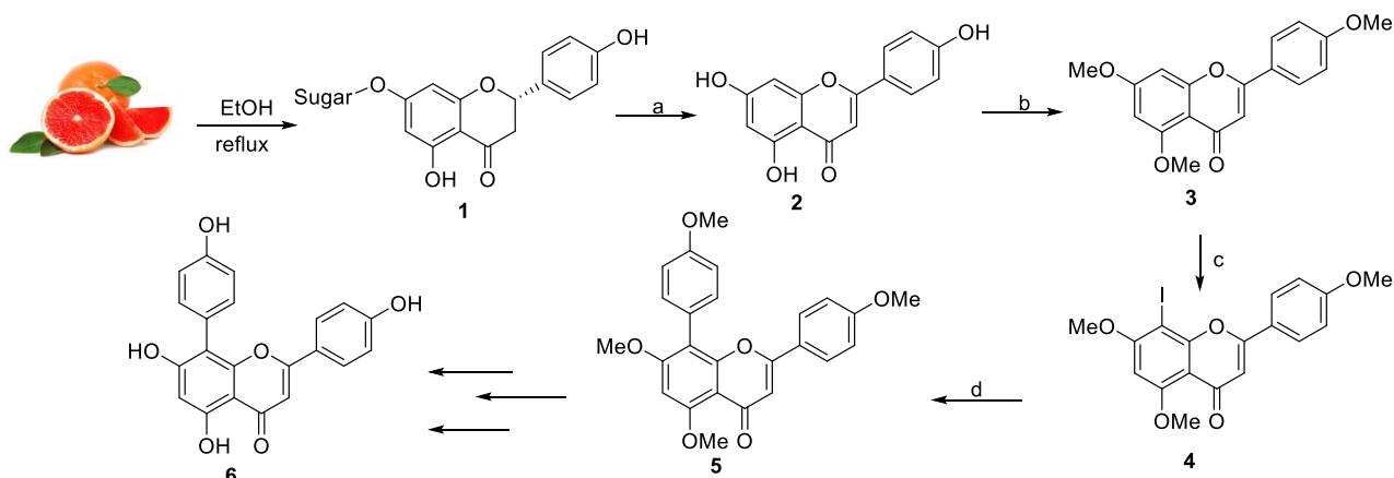
Scheme 1: Synthetic route to synthesize Podocarflavone A **6**. (a) i)  $\text{I}_2$ , pyridine,  $100^\circ\text{C}$ , 16h, ii)  $\text{H}_2\text{SO}_4$ , glycerol,  $120^\circ\text{C}$ , 1h, **74%** (over 2 steps); (b)  $(\text{CH}_3)_2\text{SO}_4$ ,  $\text{K}_2\text{CO}_3$ , acetone, 16h, **70%**; (c) NIS, DMF,  $70^\circ\text{C}$ , **65%**; (d) 4-methoxyphenylboronic acid,  $\text{Pd}(\text{OAc})_2$ ,  $\text{K}_3\text{PO}_4$ , toluene, MW,  $150^\circ\text{C}$ , 2h, **26%**.
