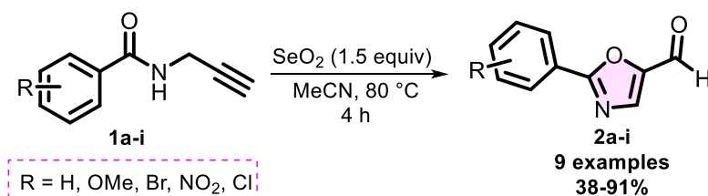
Scheme 1. Synthesis of 2-substituted oxazole-5-carbaldehydes.
