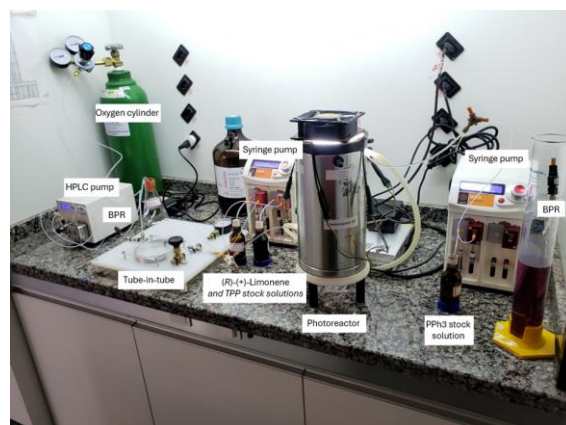
Scheme 1: Scale-up protocol for p -mentha-2,8-dien-1-ol synthesis under continuous-flow conditions. 3
